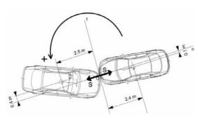
Fig. 5. The positive direction of the angle measurement relative to the x-axis of the global coordinate system and the angle of inclination of the translational velocity relative to the x axis Source: own research
