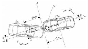
Fig. 6. Velocity components and angular velocities at the moment of collision. Also the distances from the center of the mass of each vehicle to the origin of the local coordinate system Ont are indicated Source: own research.
